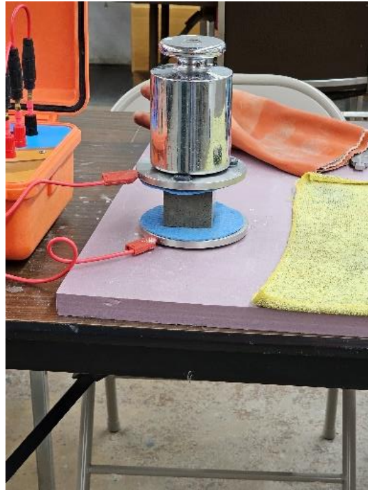
Fig. 2. Cubes tested in bulk resistivity
