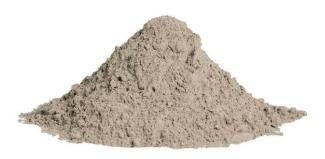
used construction materials in the world. Our Type IL is branded as **EcoCem***PLC*<sup>TM</sup> and was developed to be more environmentally friendly by reducing its carbon footprint (reduction measured through GWP). This product is a general use product for concrete and mortar as well as all the other various applications for cement, including engineered soils and solidification/stabilization of materials and wastes.
