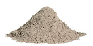
world. Our environmentally friendly product is branded as **EcoCem®PLC** and was developed to reduce embodied carbon (measured through GWP). This product is a general use limestone cement for concrete and mortar as well as all the other various applications for cement, including engineered soils and solidification/stabilization of materials and wastes.
