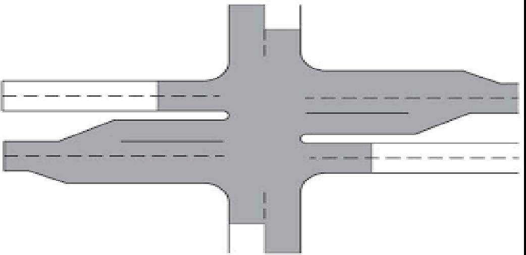
Note 1: Physical area carries the combined traffic from both roadways. Therefore, thickness design must account for both.
