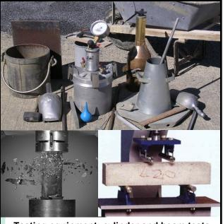
Testing equipment; cylinder and beam tests
