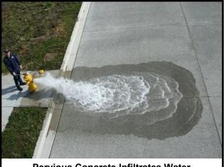
Pervious Concrete Infiltrates Water
