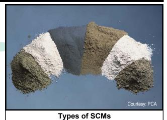
combination with cement. Slag is used at 20% to 80% by mass of the cementitious materials.
