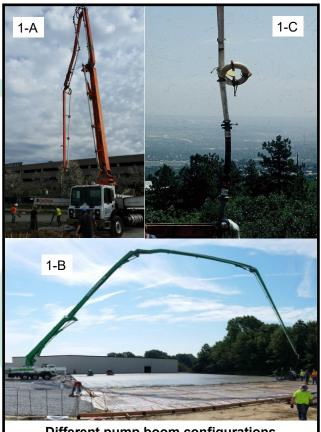
Different pump boom configurations
