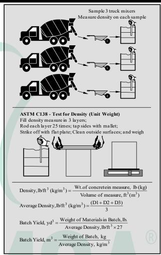
producer. Perceived discrepancies, typically underyield, is when the concrete ordered does not fill the forms due to contingencies discussed below:
