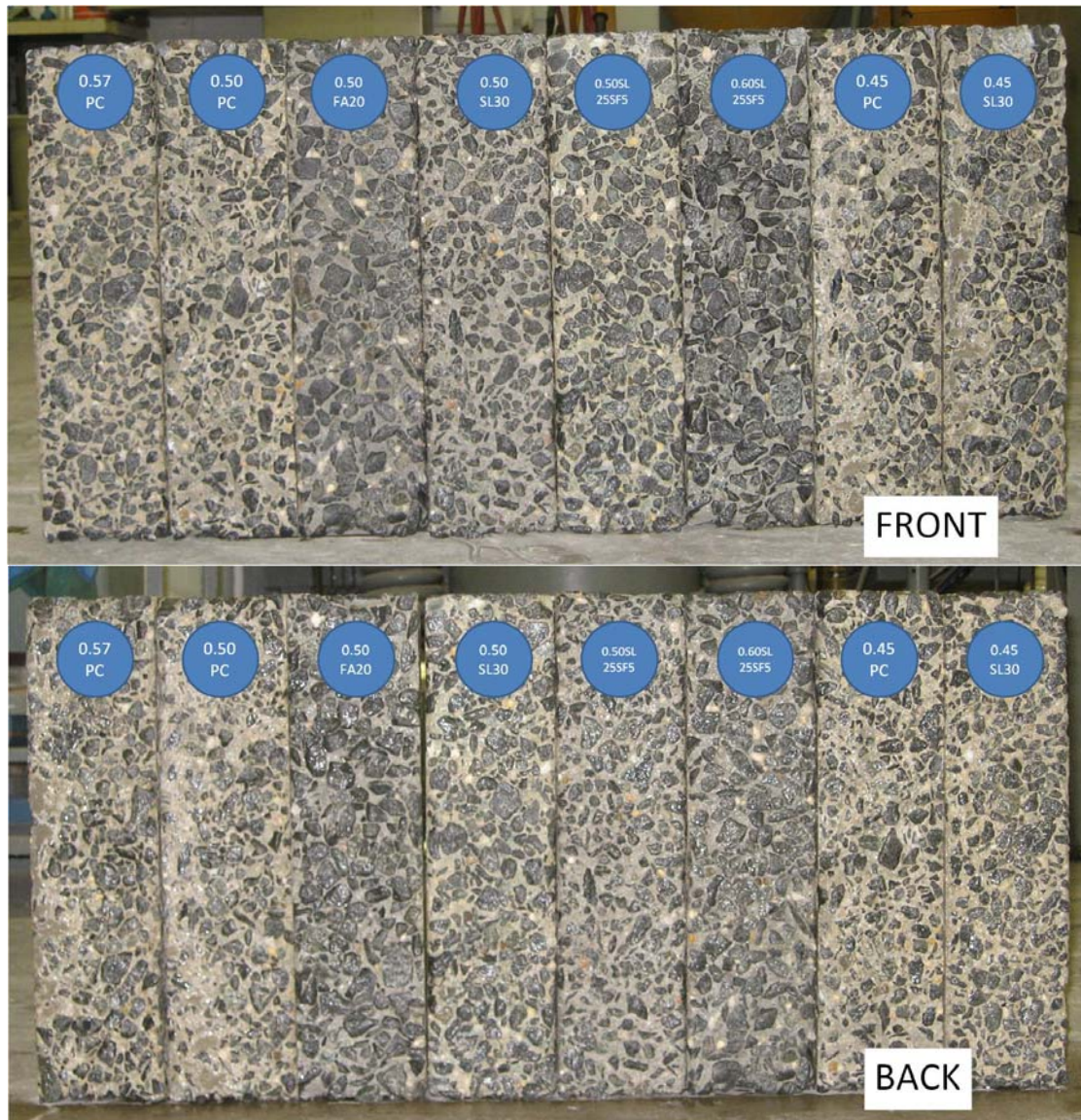
Figure 3.1 Scaling of C666 specimens After 3200 F-T cycles
