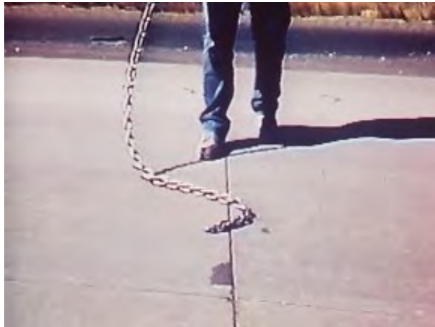
“Sounding” with hammer or chain
