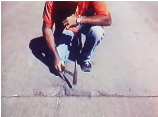
“Sounding” with hammer or chain
