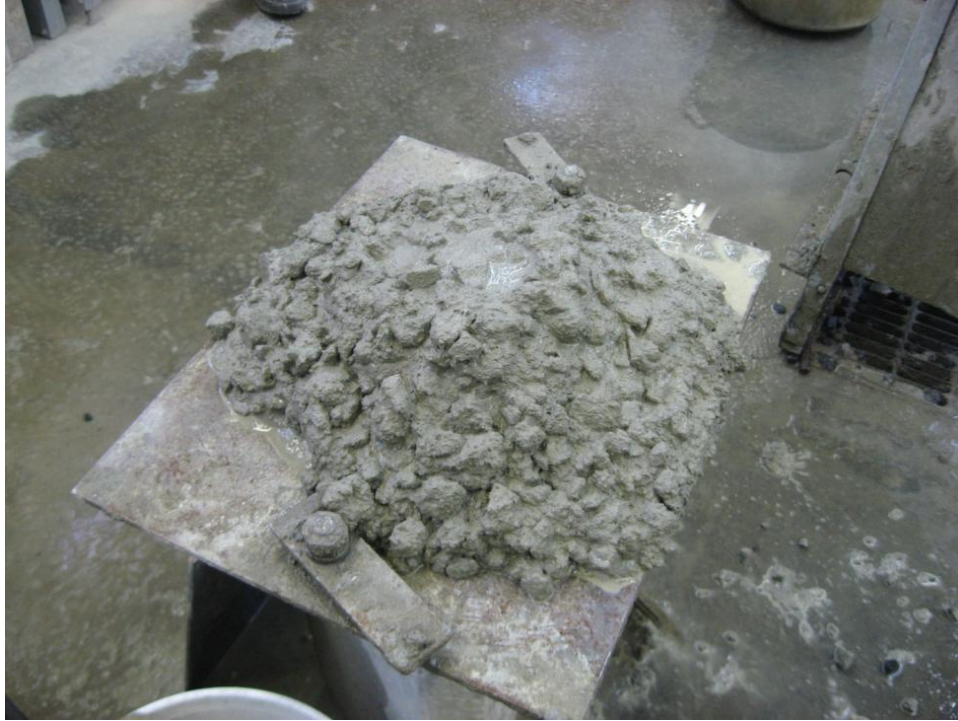
Figure 22(e) 0.40PC25 after HRWRA addition
