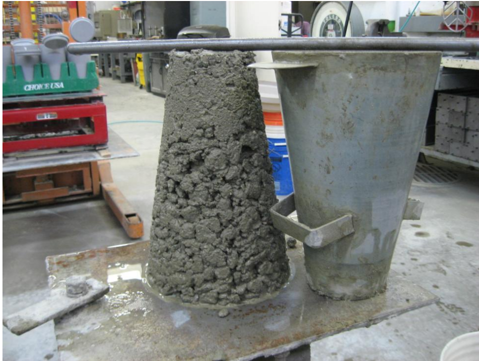
Figure 22(a) 0.55PC23 before HRWRA addition
