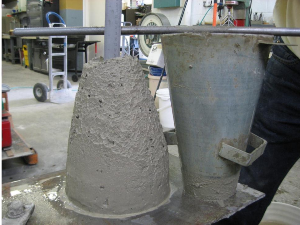
Figure 19(c) 0.47SL29A after HRWRA addition
