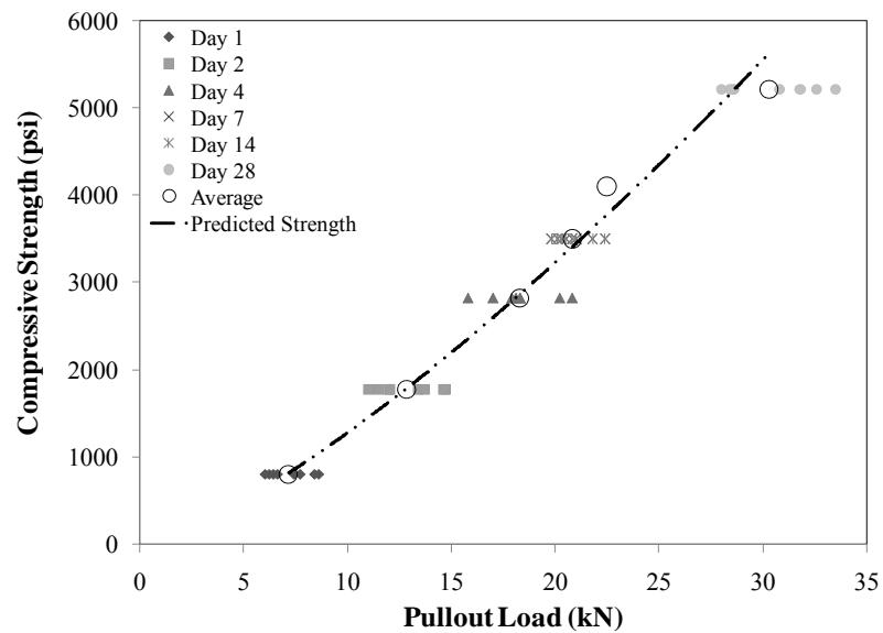
Figure D.4 Strength vs. pullout force (35% FA-C)
