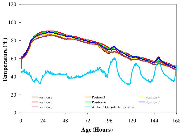
**Figure E.5 Temperature profile of block (50% FA-A)**
