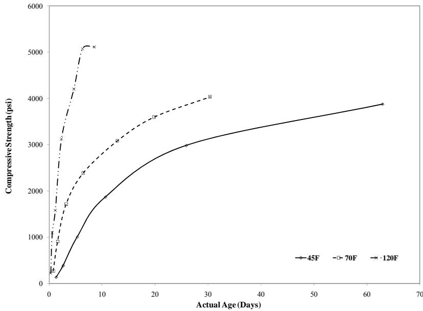
**Figure 3.4 Compressive strength vs. actual age (35% FA-C mixture)**
