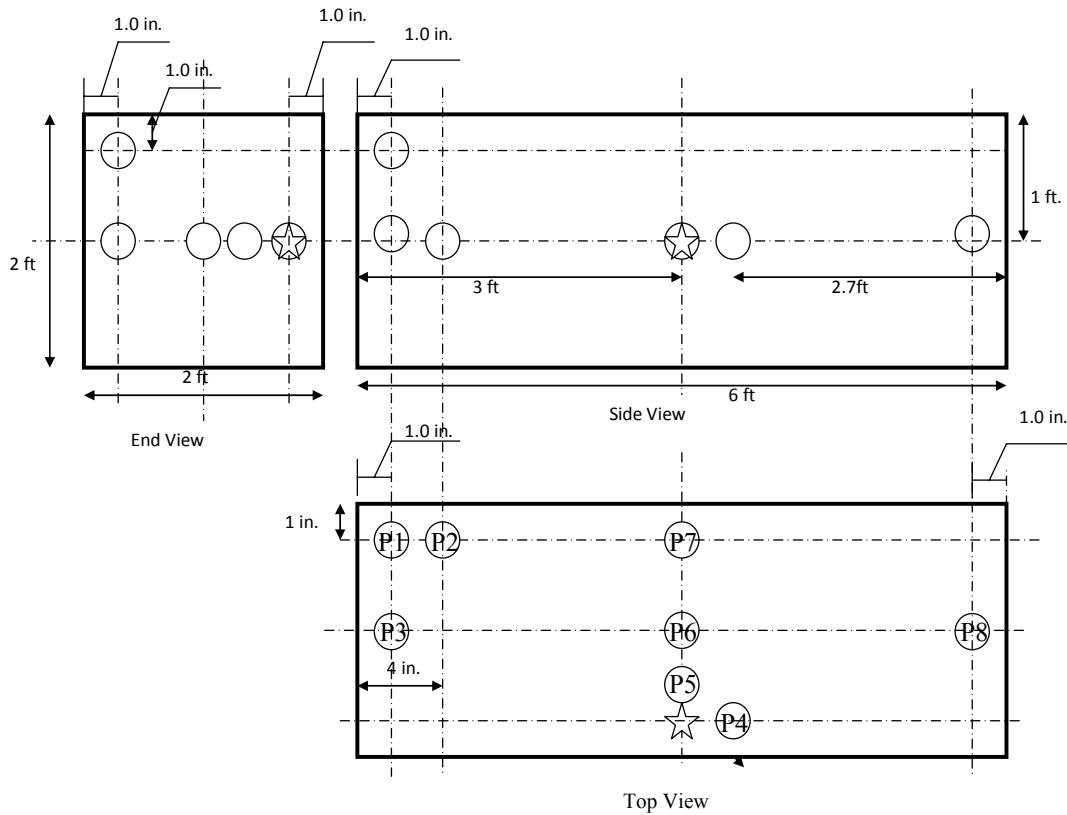
**Figure A.3 Concrete block and temperature sensor locations**
