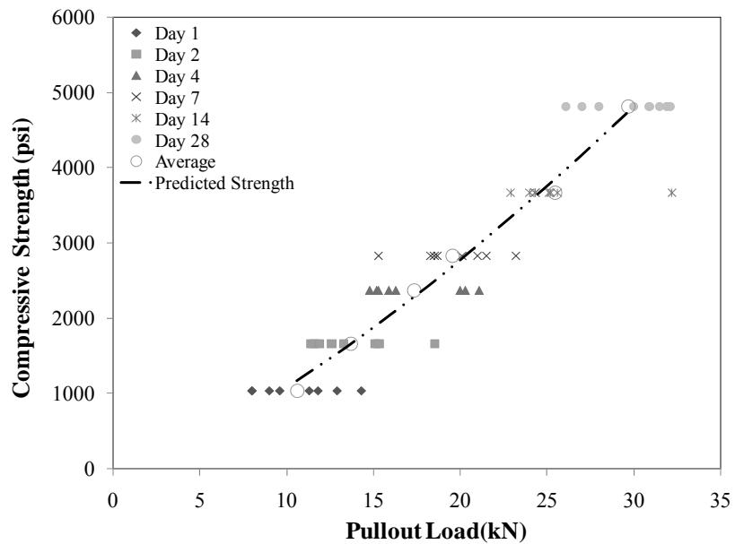
Figure D.3 Strength vs. pullout force (50% FA-A)
