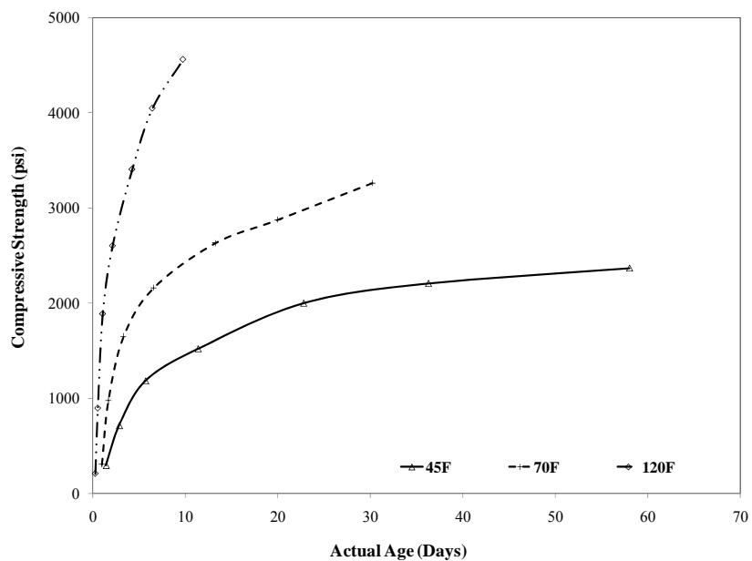
**Figure 3.3 Compressive strength vs. actual age (35% FA-A mixture)**
