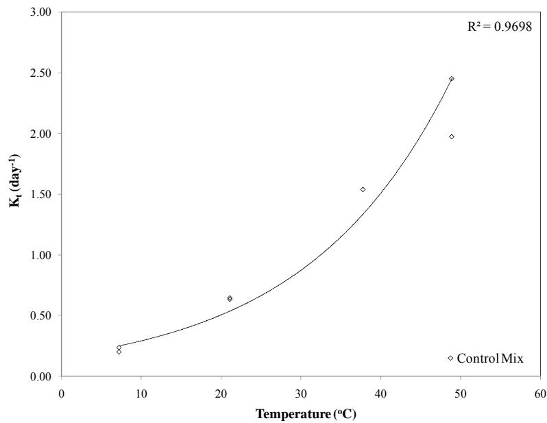
**Figure 3.5 Rate constant vs. temperature-control mixture (AE-41400 J /mol)**
