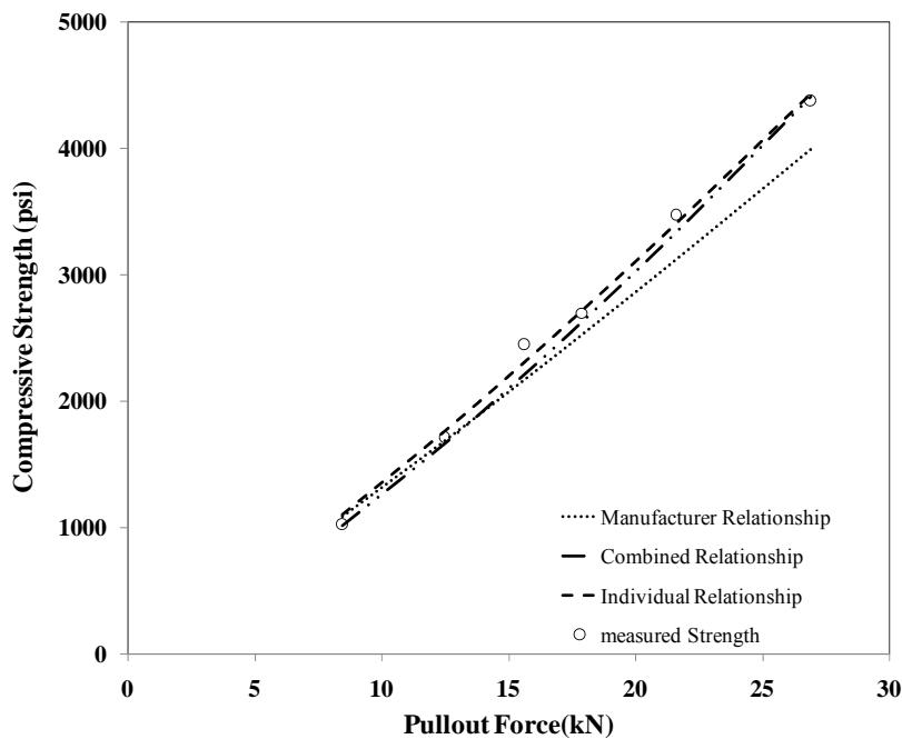
Figure 4.13 Compressive strength vs. pullout force relationship-control mixture
