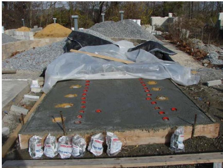
**Figure 4.8 Slabs with cast-in-place cylinders, floating inserts and field cure cylinders (The red marking are the pullout inserts, field-cured cylinders are placed outside the slab and the cast-in-place cylinders are within the slab)**
