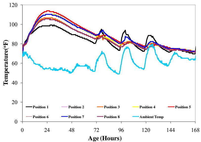
**Figure E.10 Temperature profile of block (35% FA-C)**
