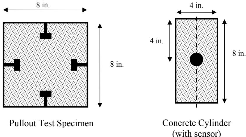
**Figure A.1 Specimens for task 3**
