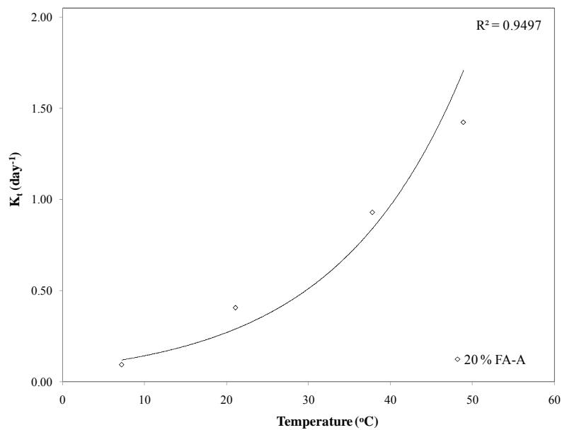
**Figure 3.6 Rate constant vs. temperature-20% FA-A (AE-48100 J /mol)**
