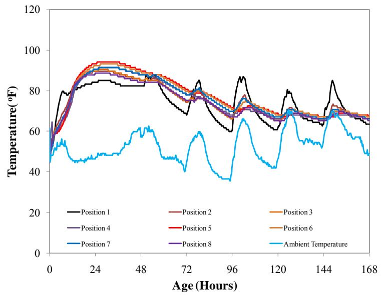
**Figure E.8 Temperature profile of block (35% FA-A)**
