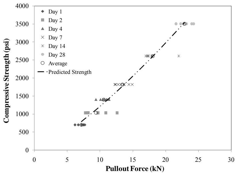
**Figure D.2 Strength vs. pullout force (35% FA-A)**
