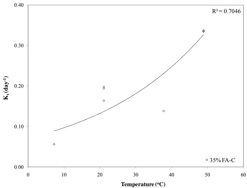
**Figure 3.10 Rate constant vs. temperature-35% FA-C (AE-28300I J /mol)**
