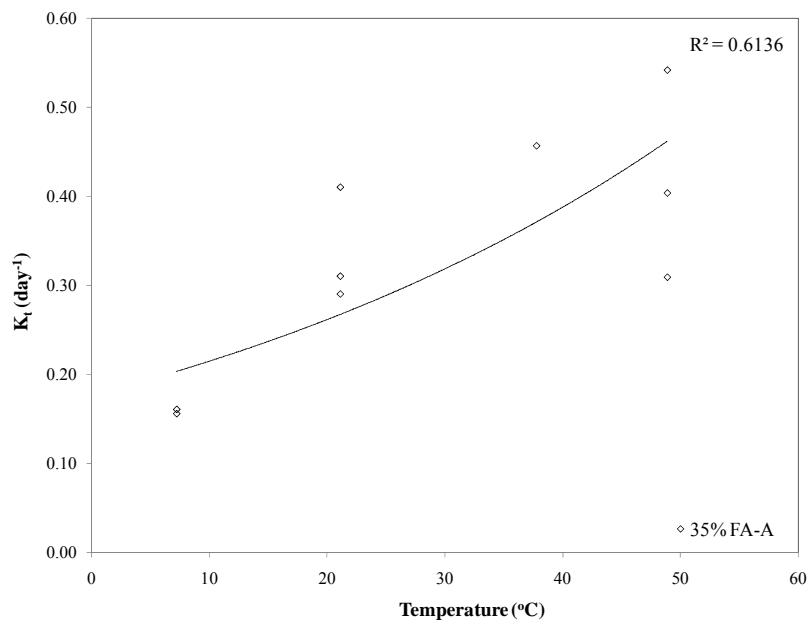
**Figure 3.7 Rate constant vs. temperature-35% FA-A (AE-15600 J /mol)**
