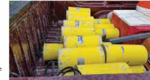
Fig. 1 Example of improper transportation of test specimens. Early-age specimens are fragile and susceptible to mechanical damage if not protected from jarring. In this example, the specimens are not restrained and can be affected by impact with each other and other surfaces. Lastly, the specimen molds lack covers for controlling moisture loss.
