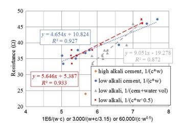
**FIG. 9** w/cm versus scaled ratio of pore solution resistivity  $(\rho_0)$  to fresh concrete resistance (R).
