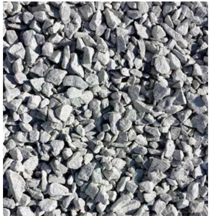
Fig 1. Aggregate that is uniform in size (gap-graded) is preferred for a pervious concrete mixture.
