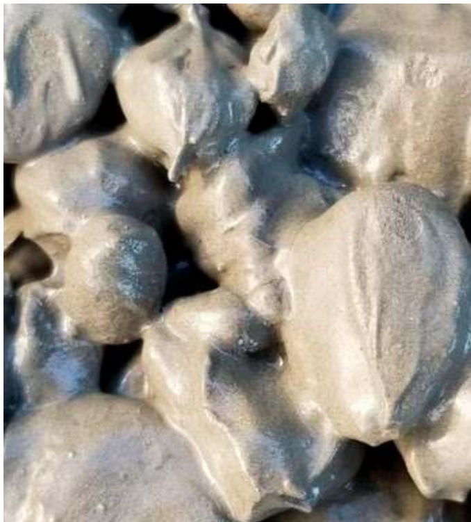
Fig 2. A properly proportioned pervious concrete mix will display a wet, metallic sheen..
