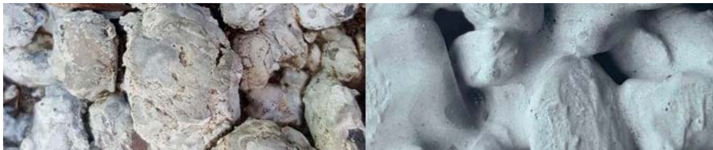
Fig 3. Un-hydrated cement causes weakness in the cement paste (left) and will significantly impact the pervious concrete's durability. A target cementitious content of 450 to 550 pounds per cubic yard, and w/c ratio of 0.34-0.41 will produce a manageable and durable pervious concrete mixture (right).
