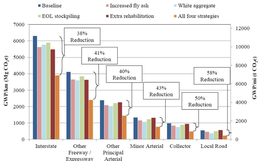
**Figure 5. GWP reduction strategies for concrete roadways using Life Cycle Assessment (LCA) methodology.**
