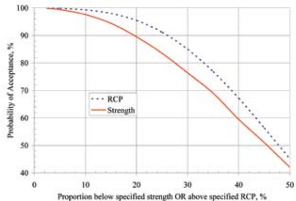
Fig. 3: Operating characteristic curves for strength (ACI 318-05 criteria) and RCP (proposed criteria)
