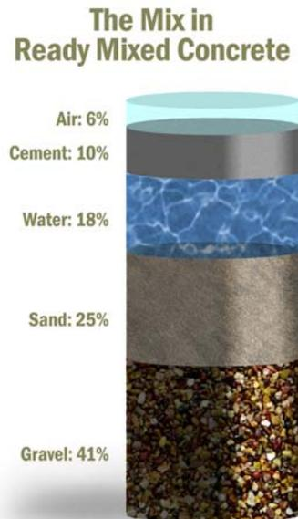
**FIGURE 2 - TYPICAL COMPOSITION OF HYDRAULIC CEMENT CONCRETE**
