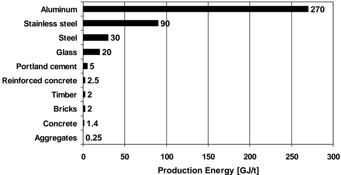
**FIGURE 3 - ENERGY OF PRODUCTION FOR CONCRETE AND OTHER COMMON BUILDING MATERIALS**
