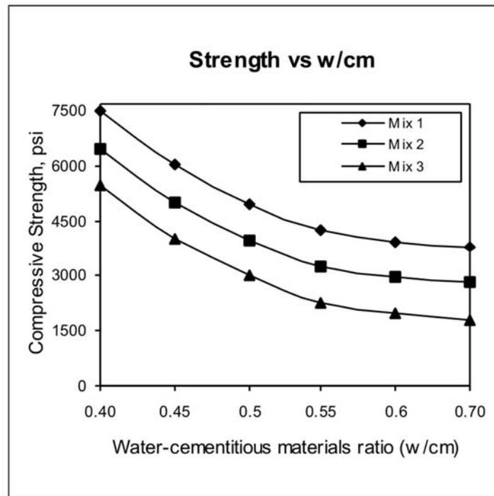
**Figure 1. W/cm alone does not control strength.**
