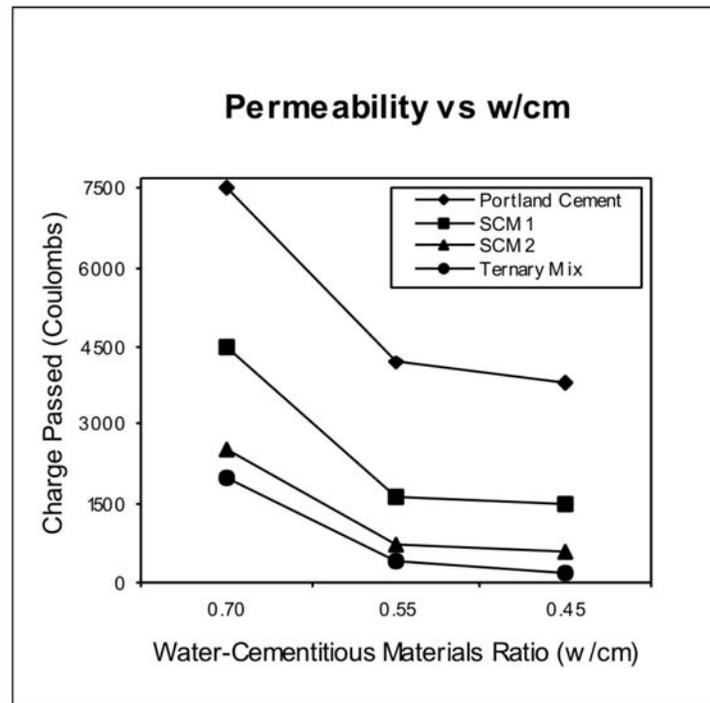
**Figure 3. W/cm alone does not control permeability.**
