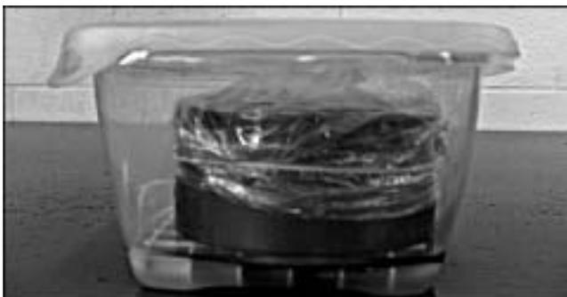
**Fig 3 Sorptivity test (ASTM C 1585) set up**
