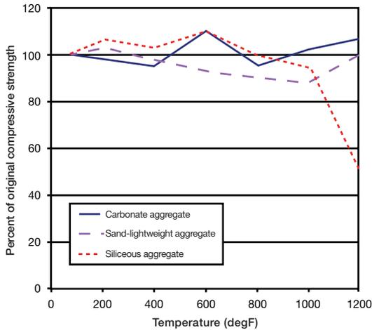
Figure 1. Strength temperature relationship for various aggregate types
