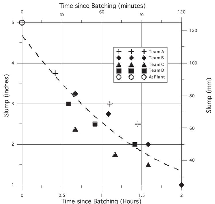
with each team spotting and correcting errors, and even with this oversight Teams A and C consistently reported the highest and lowest slumps, respectively, at any given time, with usually more than 1-inch difference from team-to-team.
