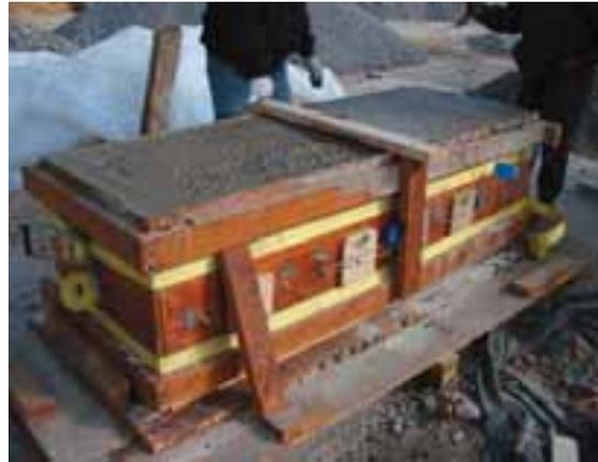
Concrete Block Cast and In-Place Strength Measured by Match Curing, Maturity, Pull-out and Field Cured Cylinders
