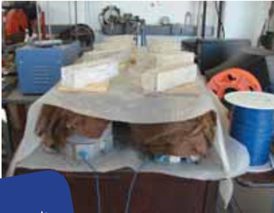
Match Cured Specimens being Cured in the Laboratory
