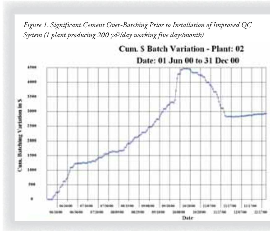
the computer properly tuned, more accurate batching was possible, as reflected by the almost flat line starting about Nov. 20.
