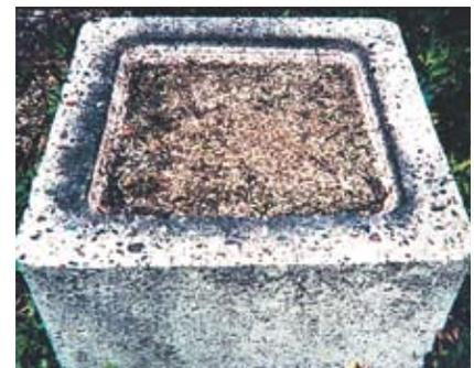
Figure 1: Damage due to exposure to freezing and thawing cycles. Courtesy Portland Cement Association.
