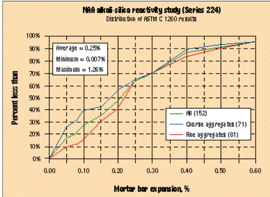
When 150 aggregate samples were tested for expansion using ASTM C 1260, only 55% of the coarse aggregates and 40% of the sands experienced less than 0.20% mortar bar expansion.
