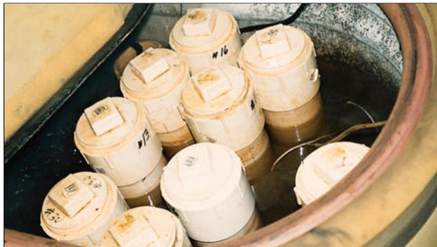
these aggregates have been used in concrete for 40 or more years. JRL technicians tested all the samples for ASR using ASTM C 1260.
