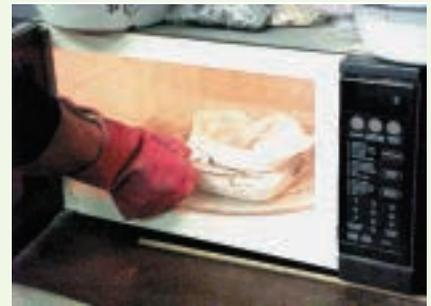
Figure 2.3 – Determining solids content in a microwave oven
