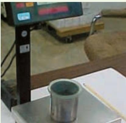
Figure 2.1 – Density measurement of water by mass
