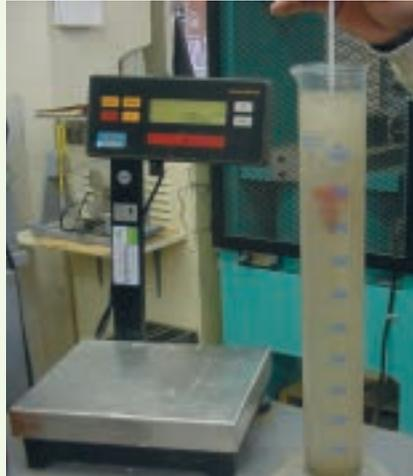
Figure 2.2 – Density measurement of water using a hydrometer
