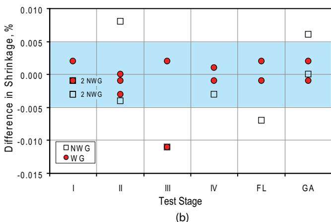
**Fig. 8: Shrinkage results for concrete mixtures produced using WG and NWG combined aggregates: (a) total shrinkage; and (b) difference in shrinkage relative to control mixture produced using NWG aggregate. Stages I, II, III, and IV represent the four stages produced at the NRMCA lab; FL and GA represent the stages produced at the Titan America Technical Services lab and Heidelberg/Lehigh Research Facility, respectively**
