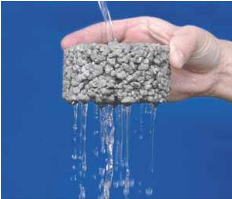
*Pervious concrete pavements help control quantity and quality of stormwater (Sustainable Sites Credit 6.1 and 6.2) and help conserve water resources (Water Efficiency Credit 1.1, 1.2, 2, and 3).*
