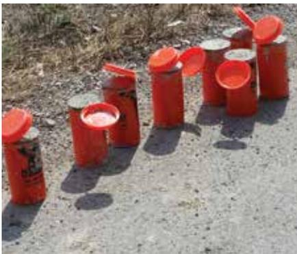
**Fig. 2:** Examples of initial curing conditions that do not comply with ASTM C31/C31M.<sup>2</sup> High temperature and moisture loss at the critical early age will lead to reductions in later-age strengths, even if standard curing is provided subsequently
