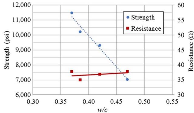
18 % and a much higher increase of about 51 % in 42-day compressive strength. For the data shown in [Fig. 4](#), linear fits to both resistance and compressive strength versus  $w/c$  yielded coefficients of determination ( $R^2$ ) that were very close to 1.
