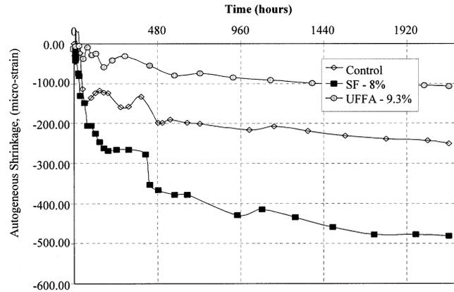
Fig. 13—Autogenous shrinkage behavior of SF and UFFA concrete.
