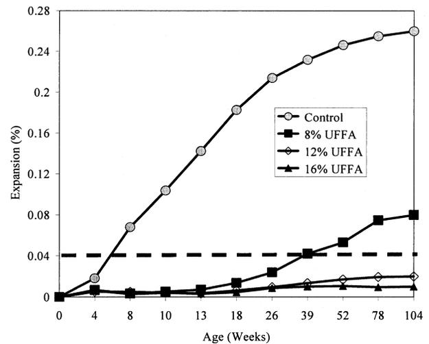
Fig. 9—Results of concrete prism test (ASTM C 1239).
