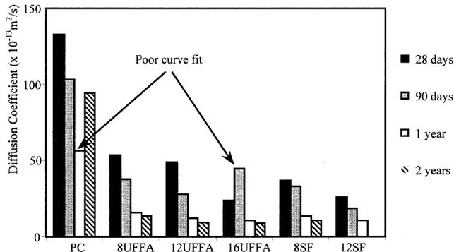
Fig. 7—Results of bulk diffusion tests.
