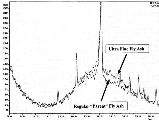
Fig. 3—X-ray diffraction data for UFFA and regular parent FA.
