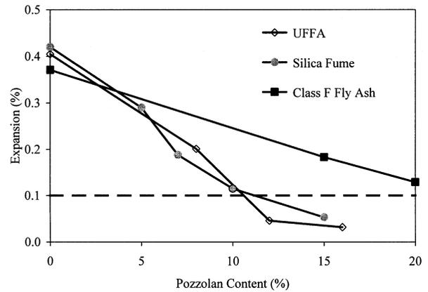
Fig. 8—Results of accelerated mortar bar test (ASTM C 1260).
