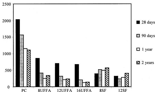
Fig. 4—RCP (ASTM C 1202) test results.
