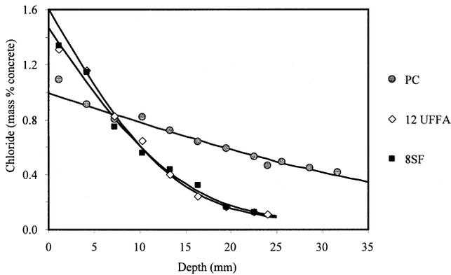
Fig. 6—Chloride profiles after 2 years of immersion.
