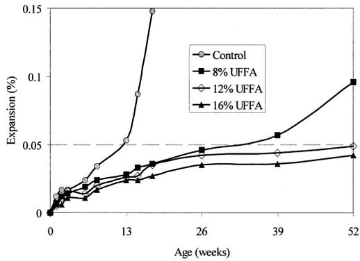
Fig. 10—Results of sulfate resistance test (ASTM C 1012).
