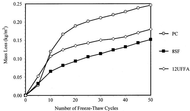
Fig. 11—Results of salt scaling test (ASTM C 672).
