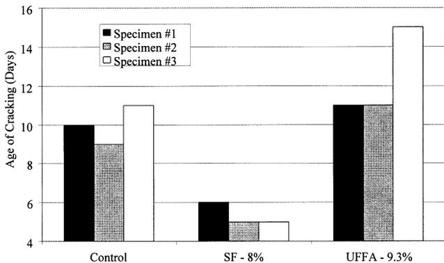
Fig. 12—Restrained shrinkage cracking behavior of SF and UFFA concrete.
