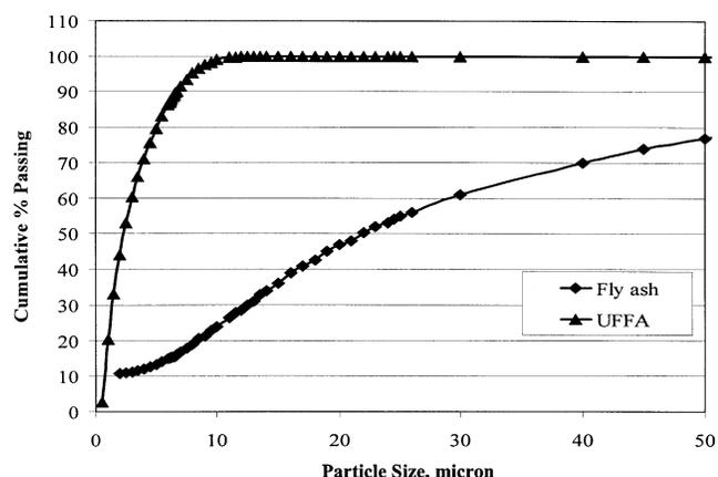
Fig. 1—Particle size distribution of UFFA as compared with regular FA.
