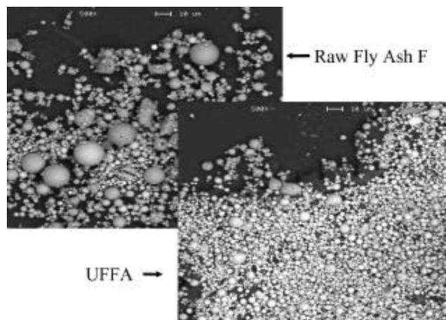
Fig. 2—SEM micrograph of typical sample of UFFA compared with regular FA.
