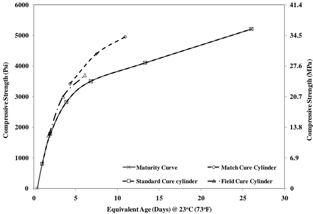
Figure 4 Compressive Strength Results for Different Curing Conditions
