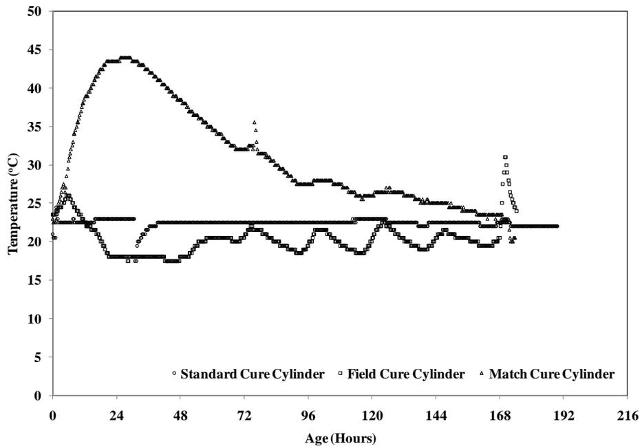
Figure 5. Thermal History of Concrete Cylinders for 35% Class C Fly Ash Concrete
