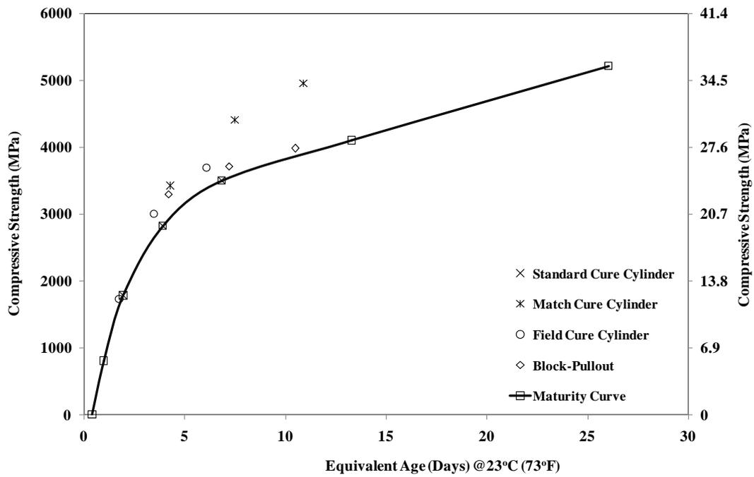
Figure 7 Compressive Strength Results versus Equivalent Age for the 35% Class C Fly Ash Concrete.
