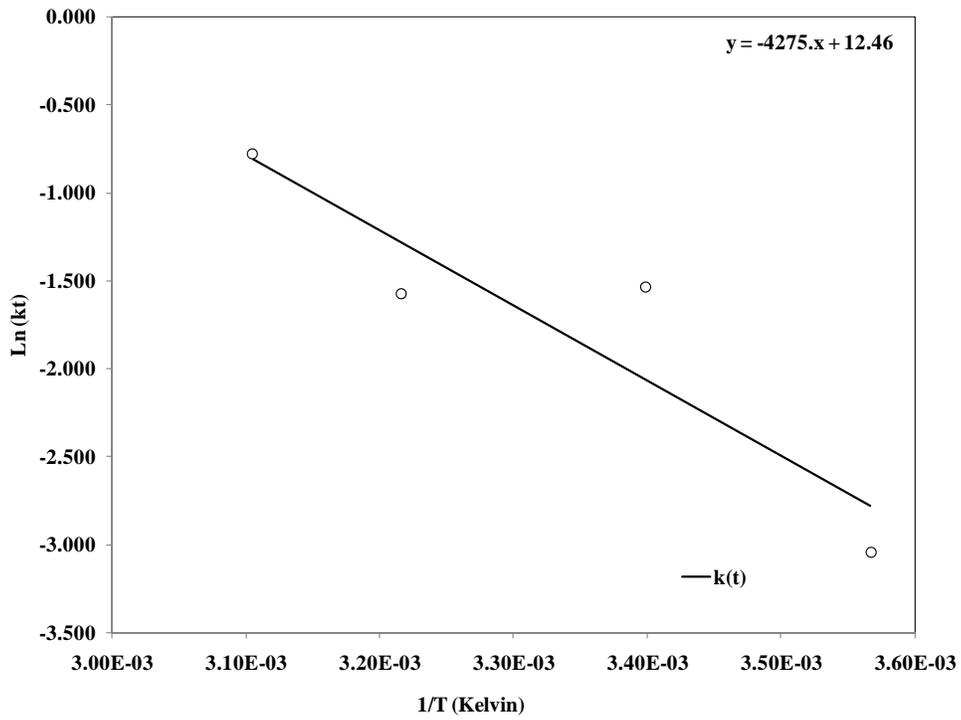
Figure 1 Arrhenius Plot for Activation Energy for the 35% Class C Fly Ash Concrete
