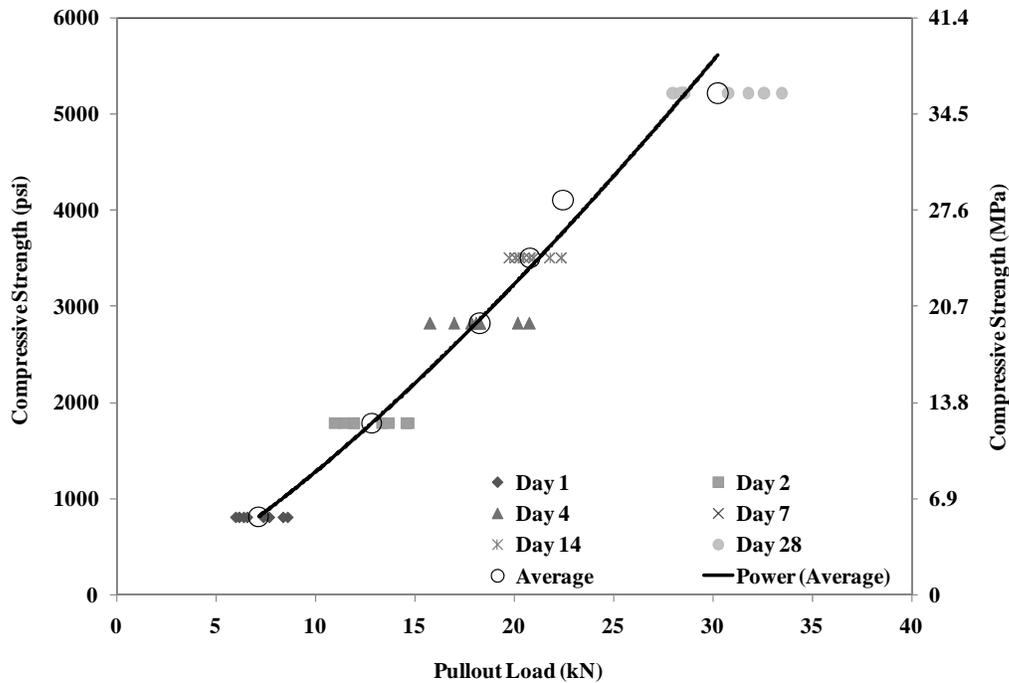
Figure 3 Compressive Strength vs. Pullout load for 35% Class C Fly Ash Concrete
