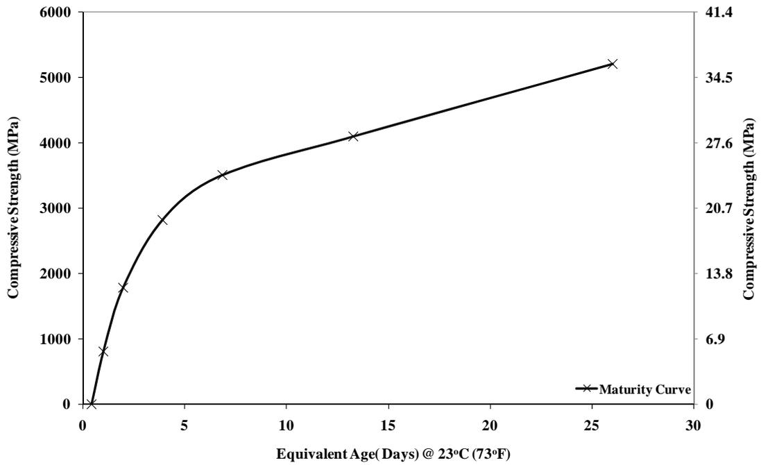
Figure 2 Equivalent Age at 23 °C (73°F) for the 35% Class C Fly Ash Concrete
