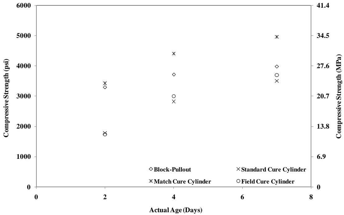
Figure 6 Compressive Strength Results from Concrete Cylinders and Pullout Test Results of the 35% Class C Fly Ash Concrete.
