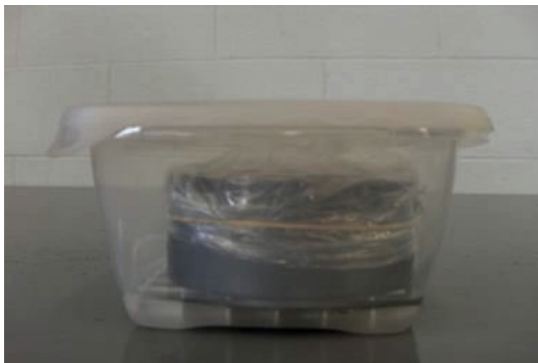
Figure 4 Sorptivity Test (ASTM C 1585) Set Up
