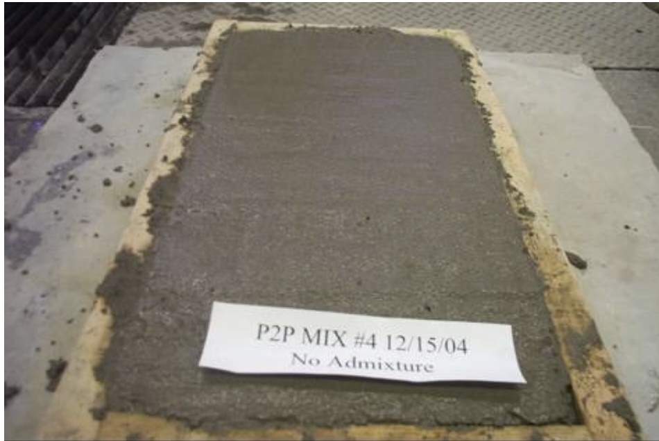
Figure 1 Finishability Test in Progress
