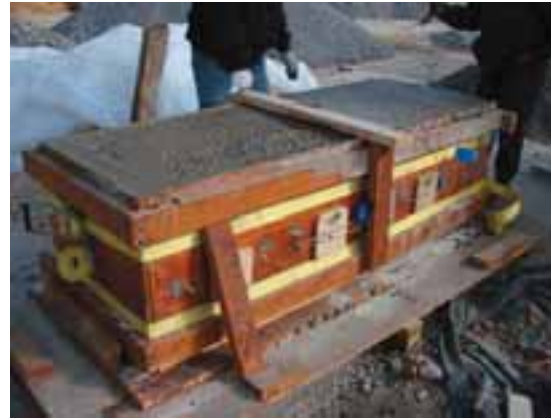
Concrete Block Cast and In-Place Strength Measured by Match Curing, Maturity, Pull-out and Field Cured Cylinders
