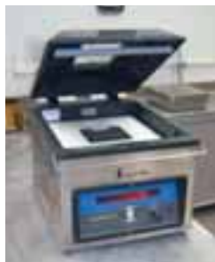
Figure 2: A Corelok system is used to vacuum air from the pervious concrete sample.
