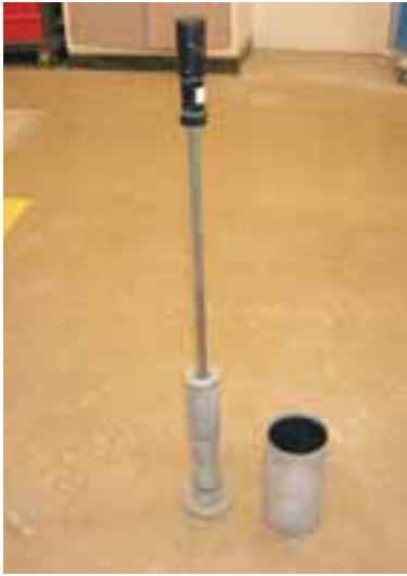
Figure 1: A Marshall hammer is used to compact pervious concrete for compressive strength testing.
