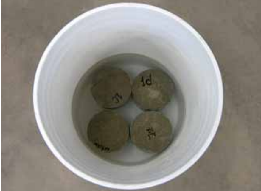
Chloride Diffusion Test (ASTM C 1556) Specimens Immersed in Chloride Solutions. (5 gallon bucket is covered and sealed until test age)
