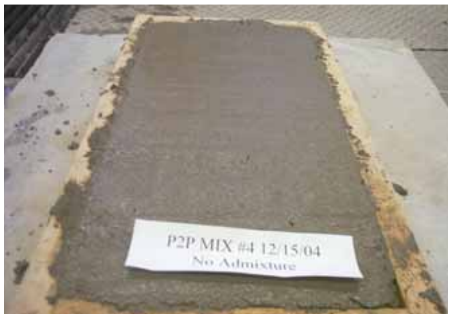
Finishability Test in Progress
