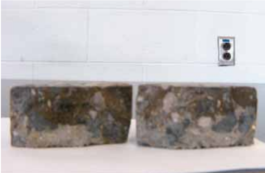
Rapid Migration Test (AASHTO TP 64) Showing Chloride Penetration Depths
