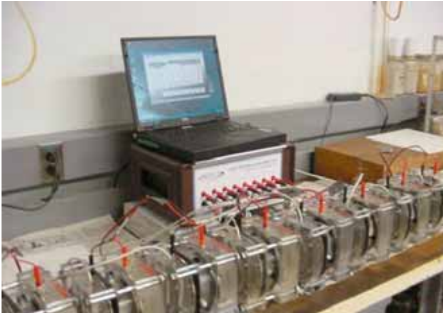
Rapid Indication of Chloride Ion Penetration (ASTM C 1202) Test Set Up
