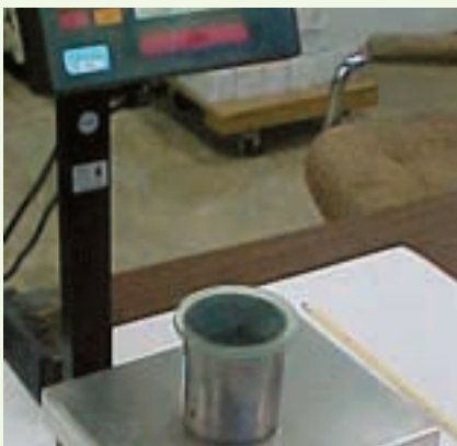
Figure 2.1 – Density measurement of water by mass
