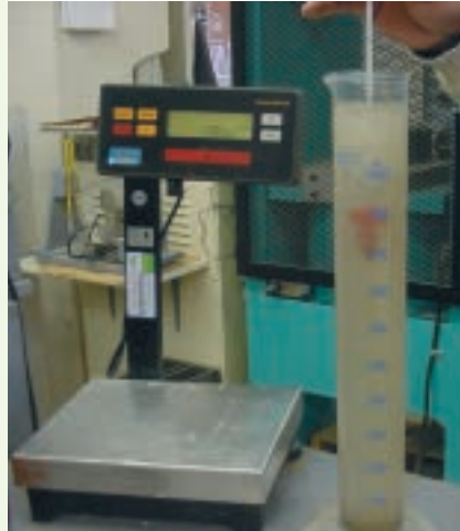
Figure 2.2 – Density measurement of water using a hydrometer
