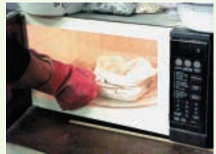
Figure 2.3 – Determining solids content in a microwave oven
