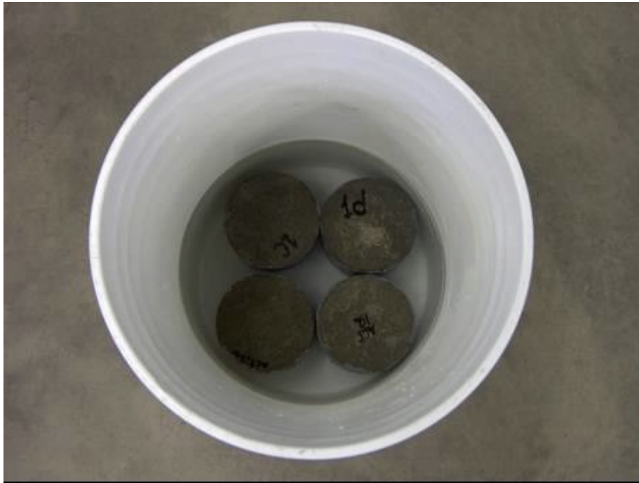
Figure 5 Chloride Diffusion Test (ASTM C 1556) Specimens Immersed in Chloride Solutions (5 gallon bucket is covered and sealed until test age)
