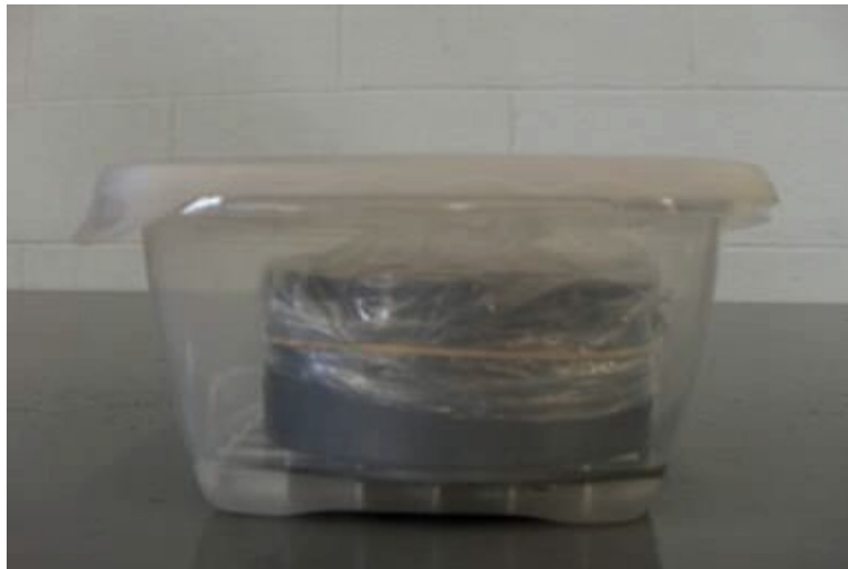
Figure 4 Sorptivity Test (ASTM C 1585) Set Up
