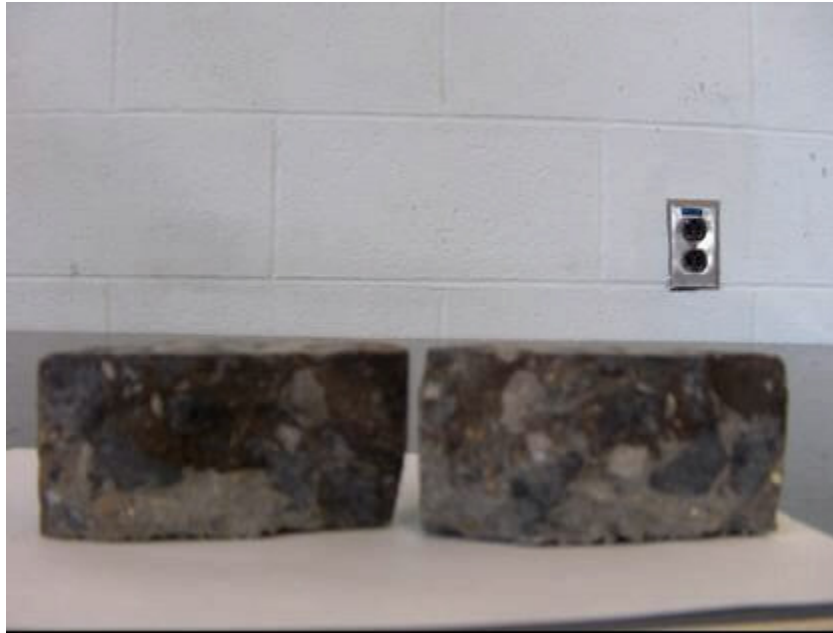
Figure 3 Rapid Migration Test (AASHTO TP 64) Showing Chloride Penetration Depths
