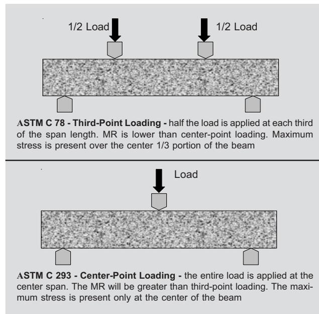
ASTM C 78 - Third-Point Loading - half the load is applied at each third of the span length. MR is lower than center-point loading. Maximum stress is present over the center 1/3 portion of the beam
